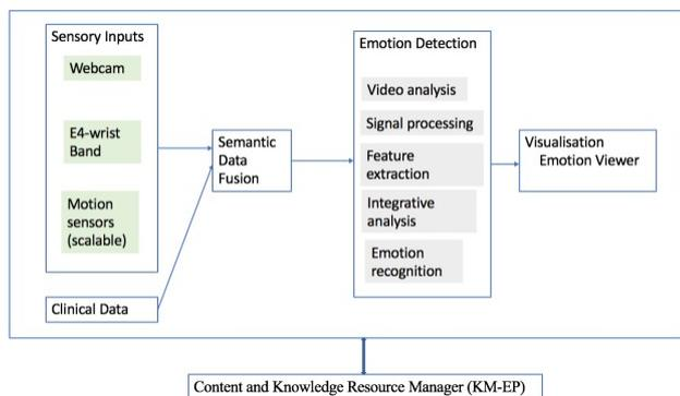
**Figure 1 SenseCare System Infrastructure**
