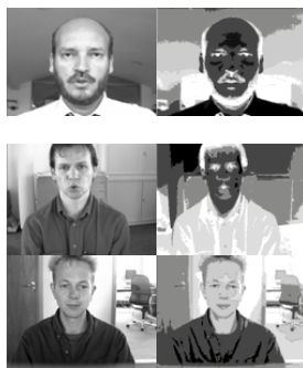
Fig. 8. Test results of face segmentation on Set 3 (BioID). (Columns left to right) Original images, Voronoi based image segmentation.
