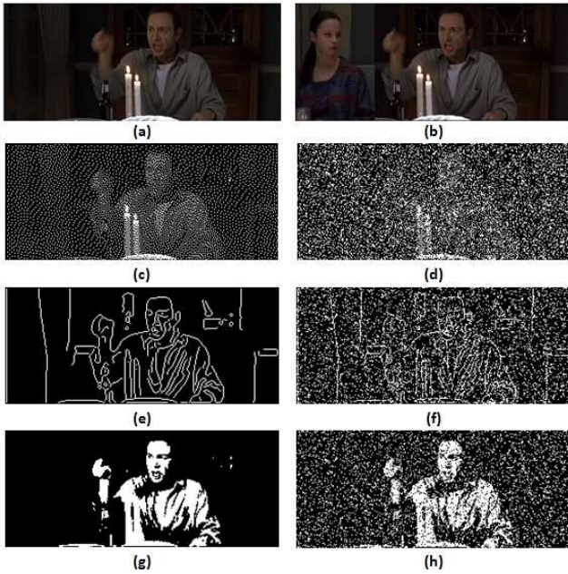
Figure 8. (a) Cover image. (b) attacked stego image. (c), (e) and (g) represent payloads and (d), (f) and (h) represent extracted payload after the spatial attack. These payloads are extracted only from attacked stego image without accessing the original image.
