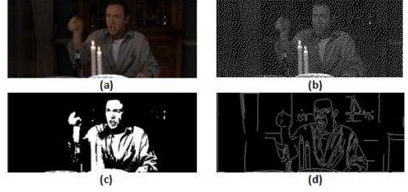
Figure 2. (a) original image. (b) created by dithering using the method described by Floyd and Steinberg [8], (c) created by thresholding the original image and (d) created by Canny edge operator respectively.
